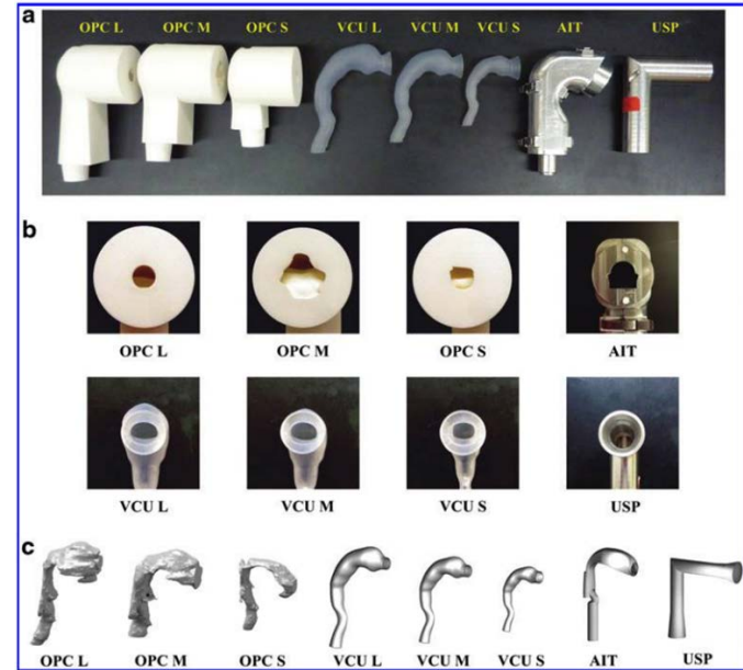
Figure 1 from Wei et al. 10 – Various realistic mouth-throat models include Oropharyngeal Consortium (OPC), Virginia Commonwealth University (VCU), Alberta Idealized Throat (AIT), and United States Pharmacopeia (USP).
