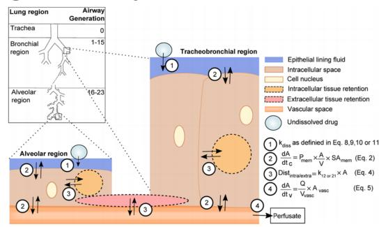
Figure 2 from Eriksson et al.<sup>8</sup> – Model structure for estimating dissolution rate constant  $(k_{diss})$  for pulmonary drug delivery.
