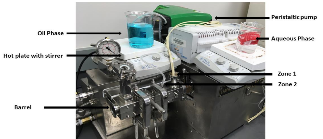
Omicron 10 [Mini] with Do/Di ratio 1.71 for manufacturing of the cream formulation. Courtesy: Steer life, USA
