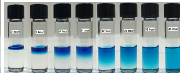
Time lapse observation of solute (methylene blue) diffusion in a_w 0.948 vehicle.-3.6 cPoise)
