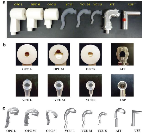
FIG. 1. Realistic MT models developed for inhaler in vitro testing: OPC Large (OPC L ), OPC Medium (OPC M ), OPC Small (OPC S ), VCU Large (VCU L ), VCU Medium (VCU M ), VCU Small (VCU S ), AIT (Medium), and USP Induction Port. (a) side view; (b) view from the mouth entry; (c) internal geometry. MT, mouth-throat; OPC, Oropharyngeal Consortium; VCU, Virginia Commonwealth University; AIT, Alberta Idealized Throat; USP, United States Pharmacopeia.
