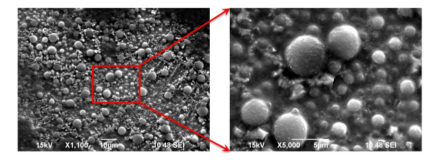
• Characteristic "honeycomb" structure not adequately observed
