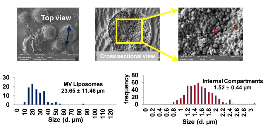
Mostly spherical shape structure; Size range of 10 - 60µm
