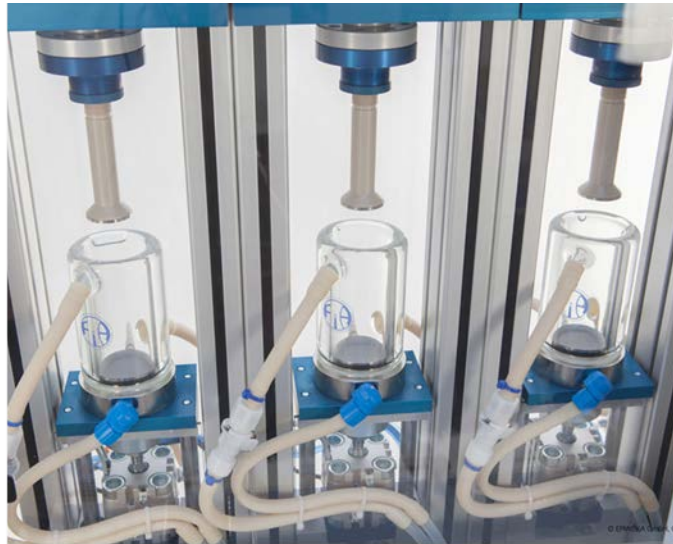
Chewing method (Erweka DRT 3 chewing apparatus, Image courtesy of Erweka)
