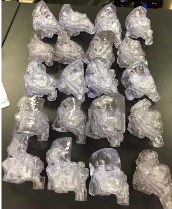
The posterior regions of the twenty nasal models printed in clear resin
