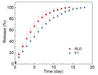
In vitro release profiles of the RLD and F1 using the USP apparatus 2 with enhancer cells with a membrane pore size of 2.7 μm). Release testing was performed in 150 mL of 1% w/v SDS in pH 7.4 PBS at 120 rpm and 37° C (mean ± SD, n=3).
