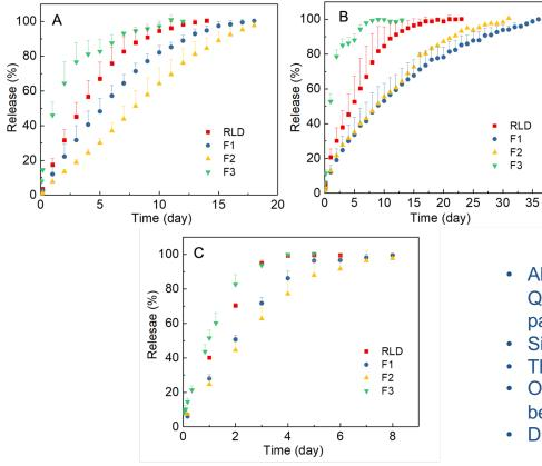
In vitro release profiles of the RLD and Q1/Q2 equivalent MPA suspensions (with different particle size) obtained using: A) USP apparatus 2 with enhancer cells; B) inhouse designed devices; and B) USP apparatus 4 with semisolid adapters at 37° C (mean ± SD, n=3).
