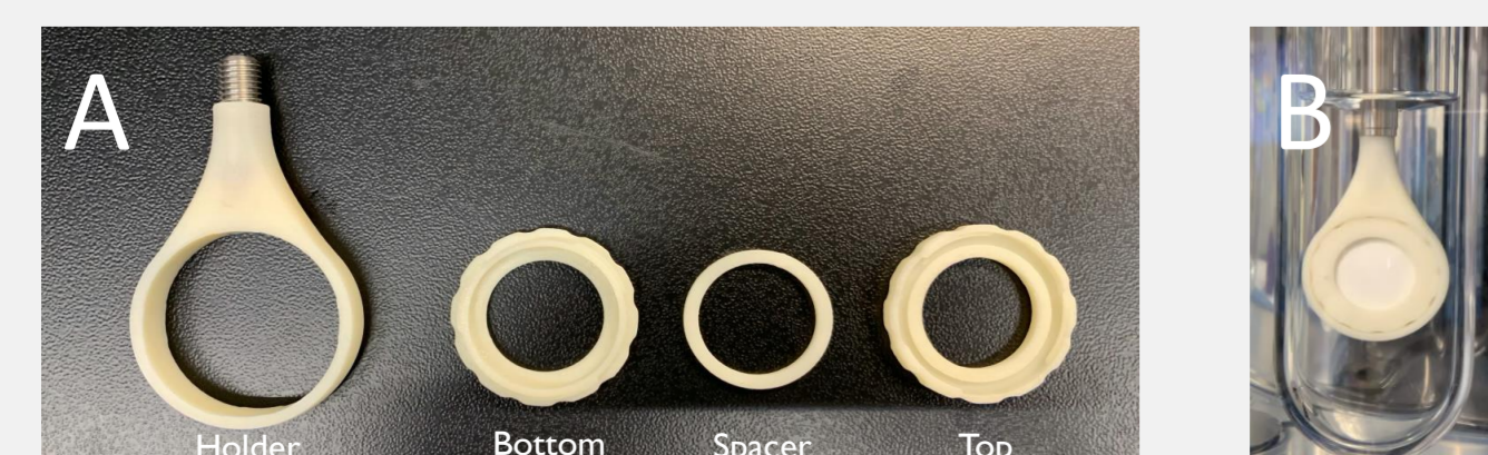
Figure 1 A: Compartments of two-sided semisolid adapter, B: Two-sided semisolid adapter in vessel
