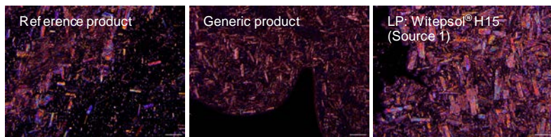
Figure 2. Polarized light microscopy images of commercial mesalamine suppositories and mesalamine in a suppository base (Witepsol® H15 Source 1). Scale bar=100 \mu m.
