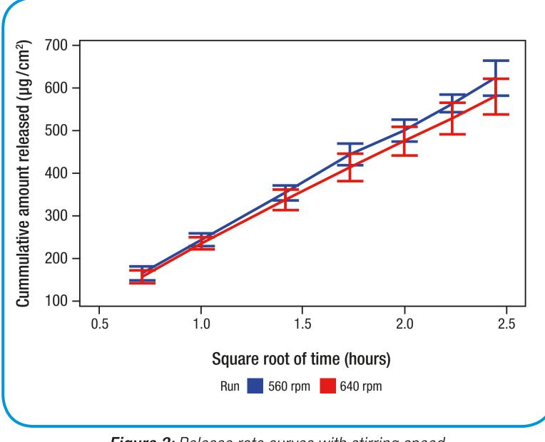
Figure 3: Release rate curves with stirring speed of 560 rpm and 640 rpm.
