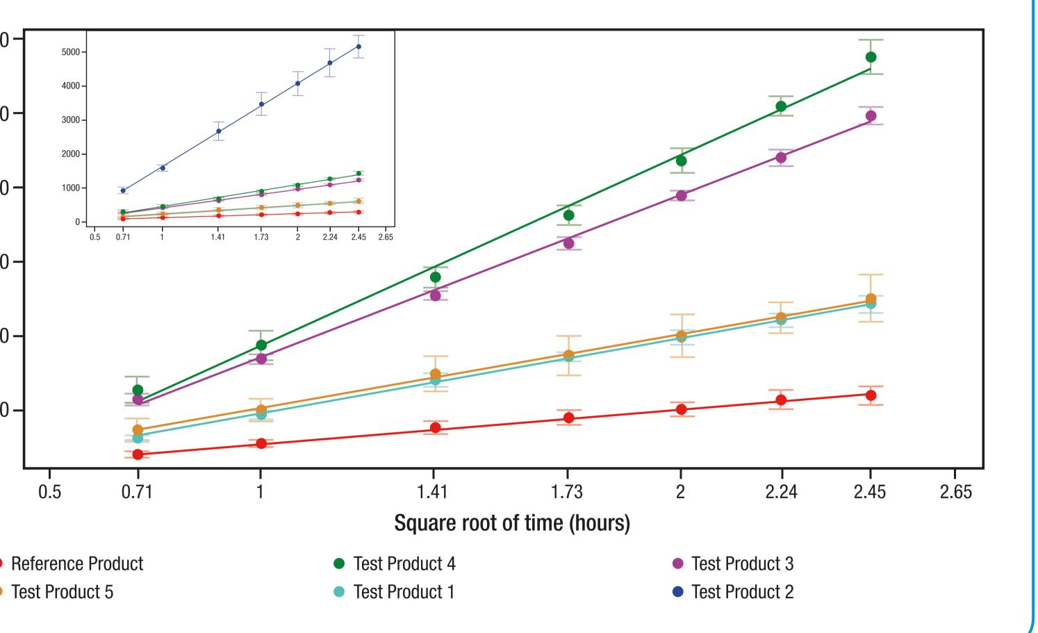
Figure 4: Release rate curves for the comparative IVRT study
