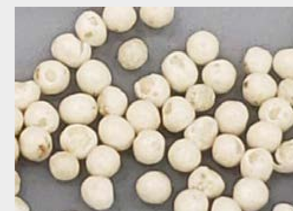
Figure 1. Photo of manipulated pellets using shaker with agate balls for 1 hours
