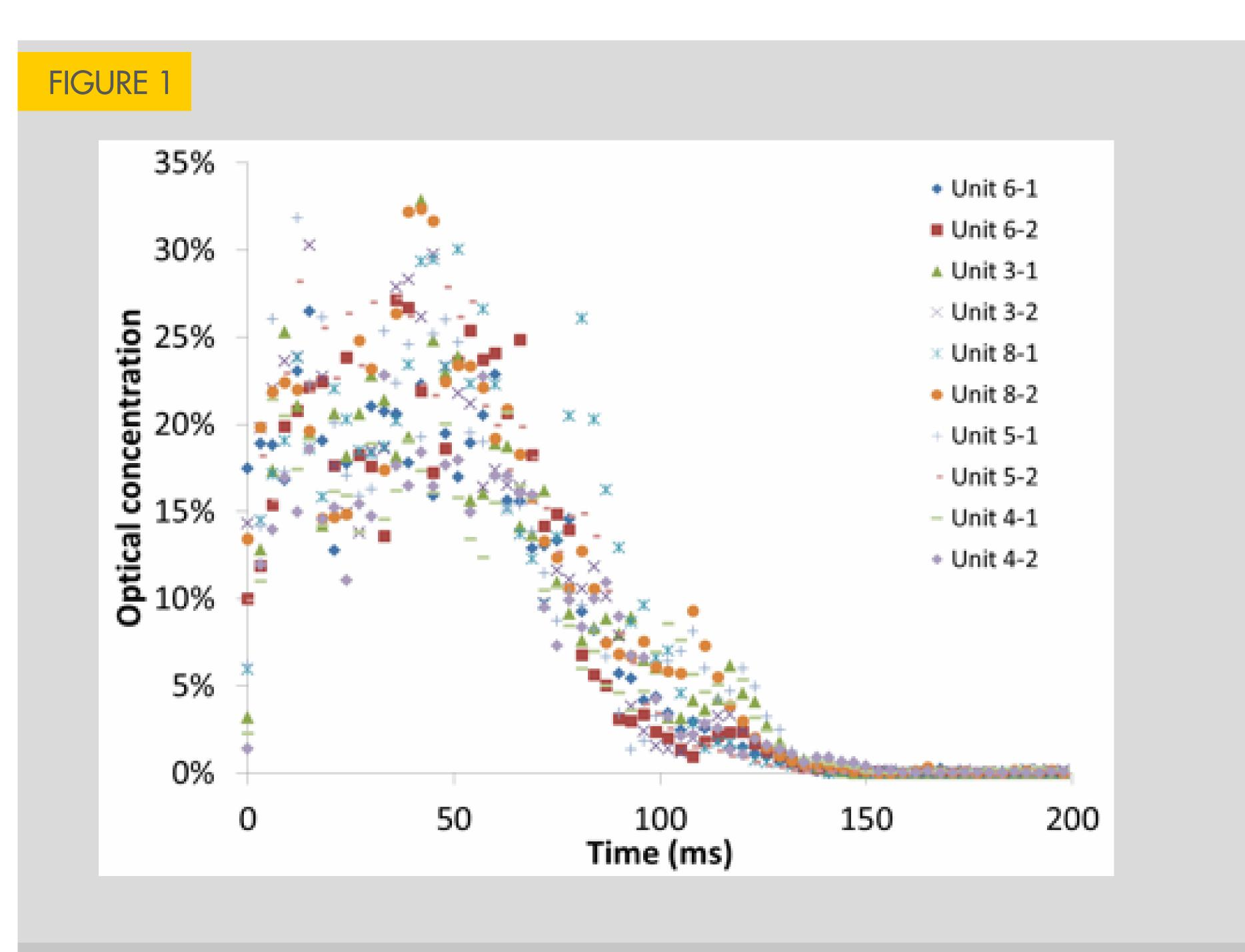
Optical concentration data from the laser diffraction measurements for the five MDIs.
