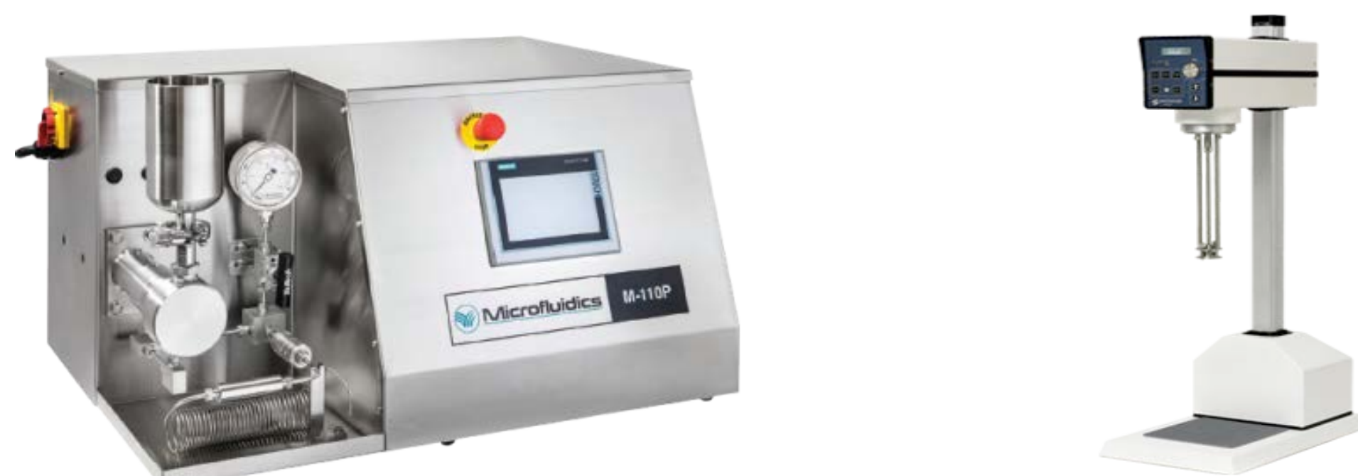
Figure 1. Microfluidization system for globule size reduction (left); and high shear laboratory mixer for generating carbomer solutions of different viscosities (right).
