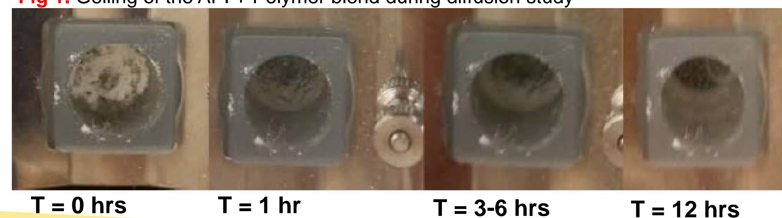
Fig 1. Gelling of the API + Polymer blend during diffusion study
